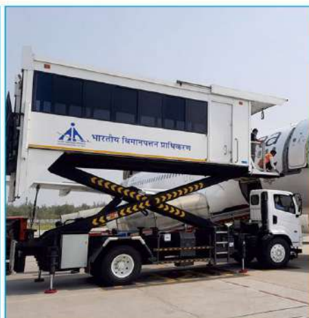
DISABLED PAX AMBULIFT Half Cabin Ambulift with Tail Lift
