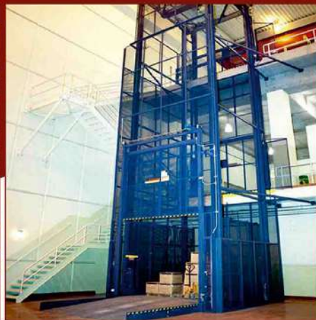
VERTICAL RECIPROCATING CONVEYOR Automated VRC to store boxes in quick manner
